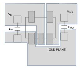
Figure 18. Layout Example for the DBV Package
