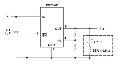
Figure 17. Typical Application Circuit
