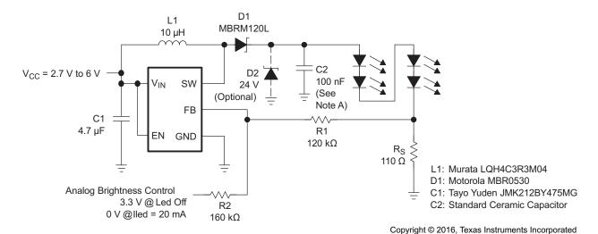
A. A smaller output capacitor value for C2 causes a larger LED ripple.
