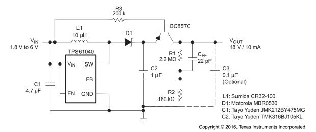
Figure 17. LCD Bias Supply With Load Disconnect
