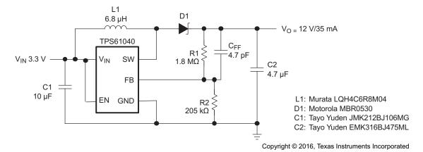
Figure 19. Standard 3.3-V to 12-V Supply
