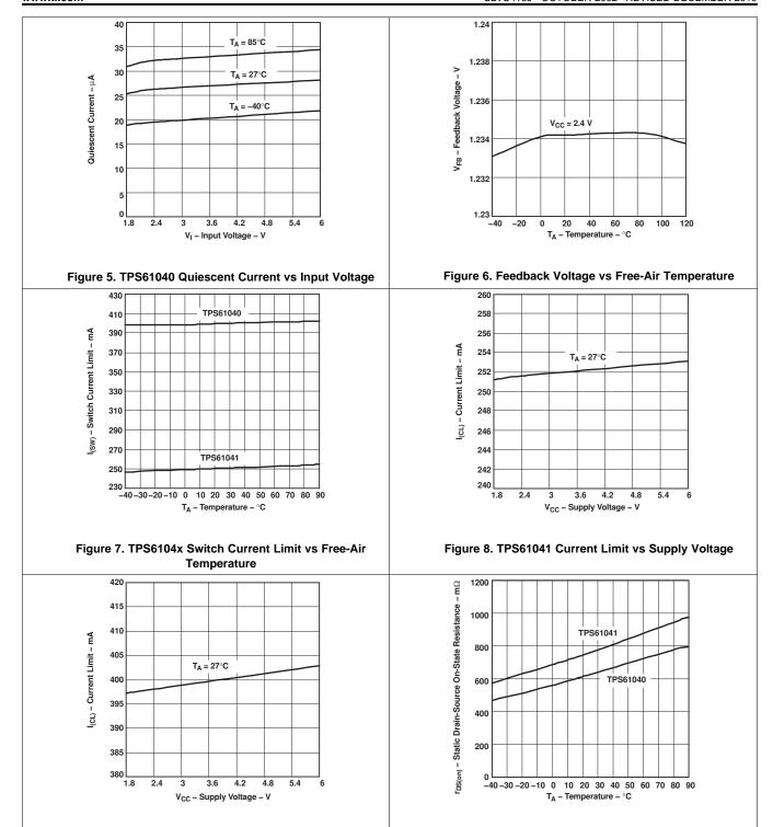
Figure 9. TPS61040 Current Limit vs Supply Voltage
