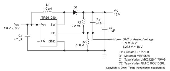
Figure 16. LCD Bias Supply With Adjustable Output Voltage
