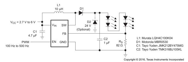
Figure 21. White LED Supply With Adjustable Brightness Control Using a PWM Signal on the Enable Pin, Efficiency Approximately Equals 86% at  $V_{\rm IN}$  = 3 V,  $I_{\rm LED}$  = 15 mA
