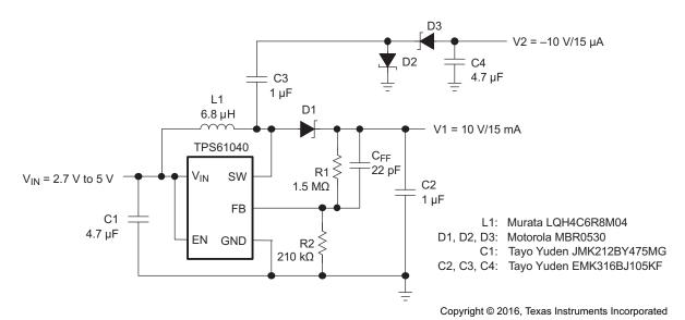
Figure 18. Positive and Negative Output LCD Bias Supply
